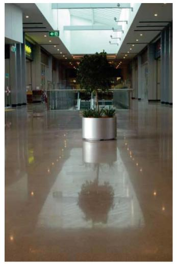
The Hiperfloor<sup>TM</sup> process transforms already existing concrete substrate into wear resistant, beautiful floors. This reduces the requirements to install other surface treatments.
